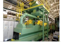
Tumbler Shotblasting Machines are suitable for blasting of mass produced components similar shapes and sizes. Mostly used in steel, gray-iron, nodular, aluminum foundries and for forgings.
